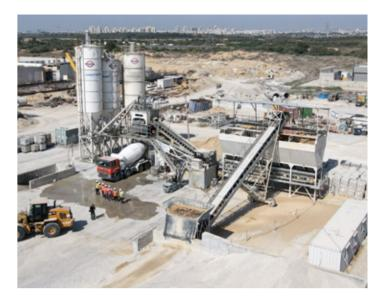
In the wet production method, the various components are poured through a sealed system into a mixing chamber, which then pours it ready-made into the concrete truck. In this process, no pollutant particles are emitted into the air, and the truck engine is not ramped up, sparing significant noise nuisance. In addition, the Electra Infrastructure concrete plants use mainly washed/rinsed raw materials that contain a low ratio of airborne particles.
